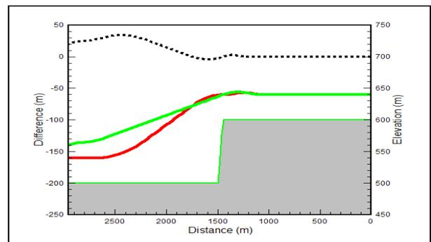
**Figure 4.** Simulation of vertical flight path for opposing flight line directions over a 100m cliff
