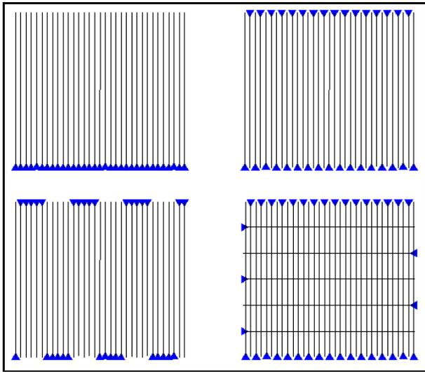
**Figure 2.** Examples of simulated flight line directions needed for realistic construction of survey models. The examples show constant, alternating, racetrack and tie line configurations.
