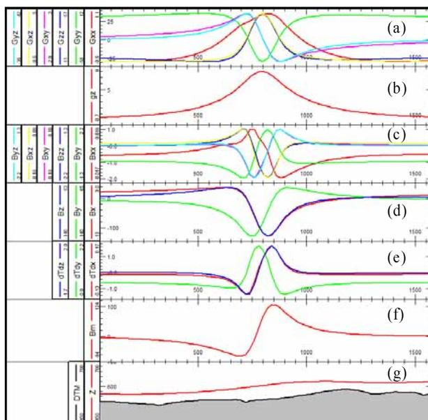
**Figure 6. A comparison of sensors over the dyke shown in Figure 5 showing the gravity tensor (a),  $G_z$  vertical component of gravity (b), magnetic tensor (c), magnetic components (d), total magnetic field gradients (e), total magnetic field (f) and flight path over terrain (g).**
