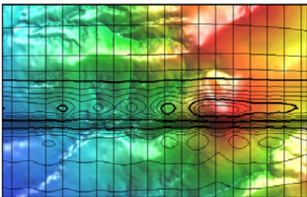
**Figure 5b. Contours of the gridded magnetic data from the simulated alternating heading direction survey superimposed on a pseudocolour image of the terrain. The contour closures result from variable terrain clearance over the dyke.**
