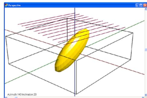
With ModelVision, you can now use the joint inversion with gravity gradiometer data or cross-wing magnetic data to better resolve the depth, dimensions and attitude of a deep IOCG deposit. You can use both methods together in the form of cooperative inversion as IOCG deposits usually have a high density and high magnetic susceptibility. This process is applied sequentially to each data type using the same model for each joint inversion.
